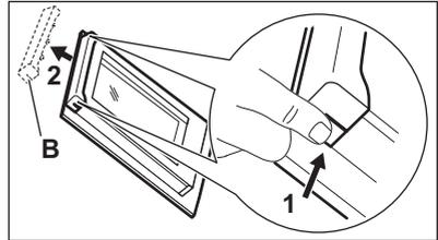
**Step 7** Hold the door glass panels by their top edge and carefully pull them out one by one. Start from the top panel. Make sure the glass slides out of the supports completely.
